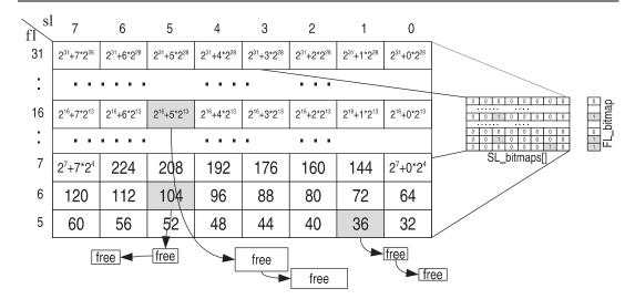
Figure 5. TLSF data structures example.
