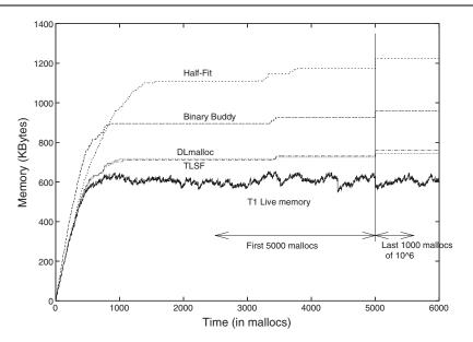
Figure 9. Memory used during one of the simulations of profile 3.
