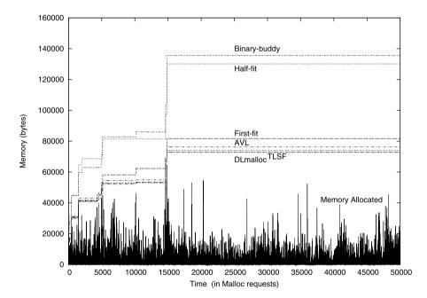
Fig. 5 Evolution of the memory required by each allocator
